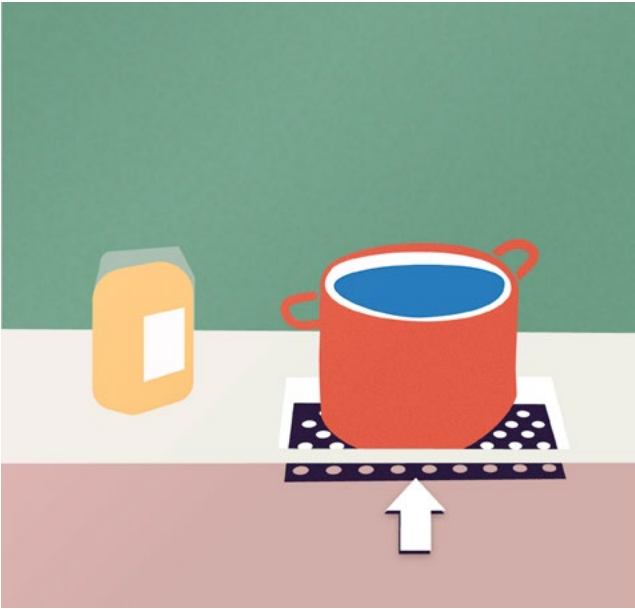
The bottom of your sink rises automatically to the same level as the worktop so that you don't have to lift the pot.
